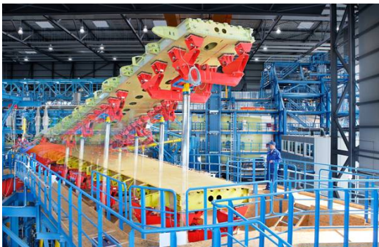
Structural airframe testing (e.g. A380)
